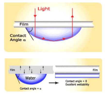
The droplets formed on the film's surface cause internal reflections of light and as a result fogginess develops.
